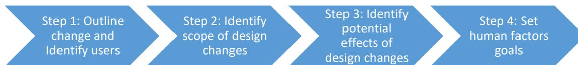
Figure 2: Steps in the Human Factors Impact Assessment tool for Railway Change Management
