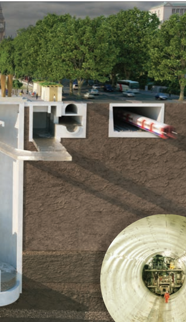
● Cross section of the Thames Tideway Tunnel
