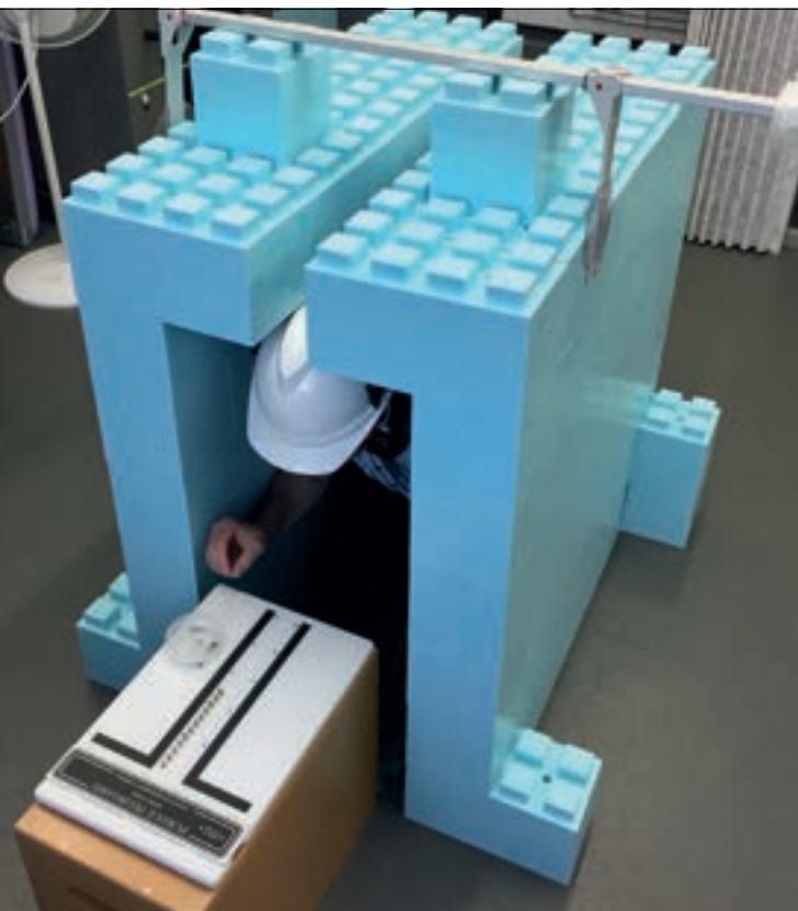
● Trialling the test conditions for a Purdue pegboard test in a restricted space
