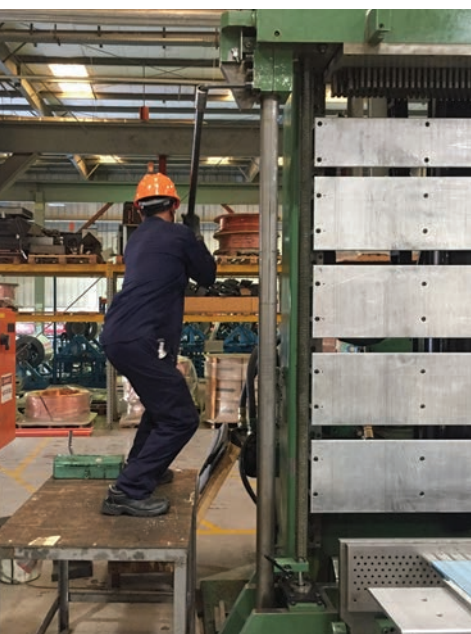
Worker adjusting a bolt torque on an expander machine
