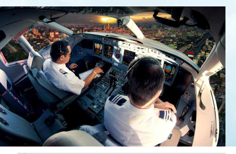
usage of the aircraft. During simulator training, pilots learn how to handle technical problems or 'abnormals' with the help of the ECAM or EICAS.
