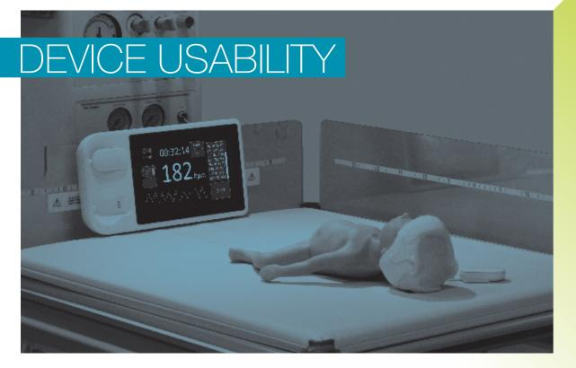
THE PROBLEM: A new device had been developed to assess heart rate during resuscitation of newborn babies, to ensure clinicians are provided with accurate information in a timely and precise manner, without the need to stop resuscitation for manual heart rate assessment with a stethoscope. What information is needed for such as device and how should it be displayed and controlled?
