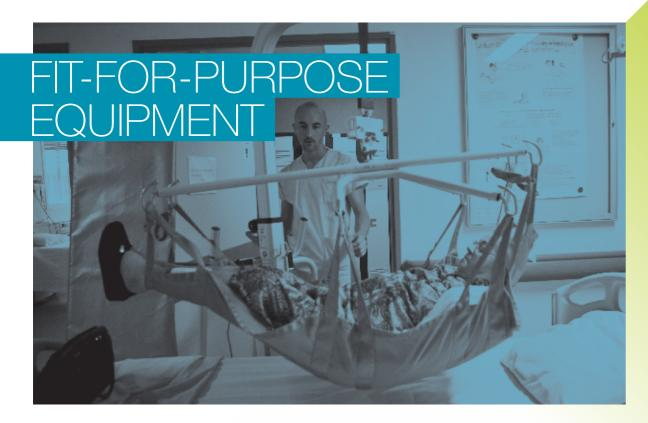
THE PROBLEM: Carpeted floors in a newly-built hospital prevented easy use of a mobile patient hoist. The hoists were a control measure implemented to reduce the risk of manual handling injuries to staff. The hoist's rubber wheels worked well on smooth or hard floors but not on carpet. When a patient was in the hoist, the wheels sank into the carpet, making it difficult to move so nurses stopped using them, increasing the risk of injury to staff and patients.
