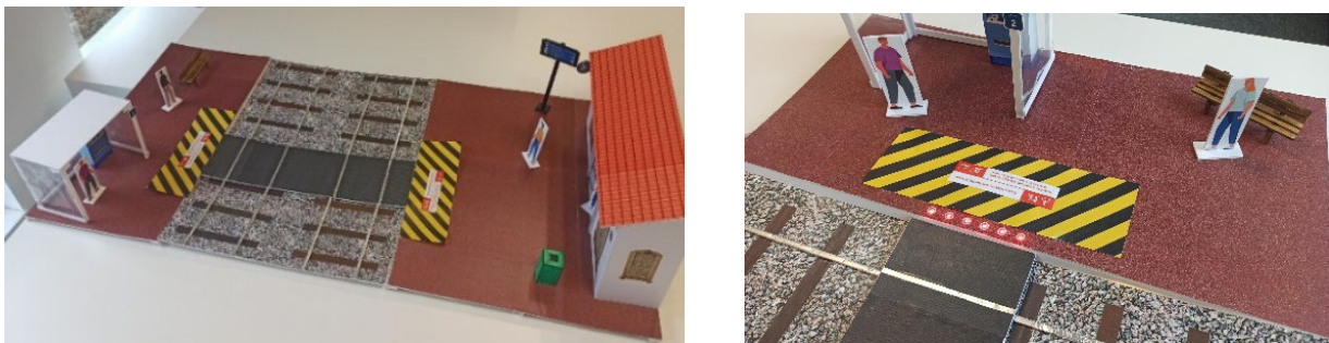
Figure 1: 3D-reduced model of a train station composed of two platforms, a portion of a double-track railway, a SPC (left); model of a safety device element shown activated (right).
