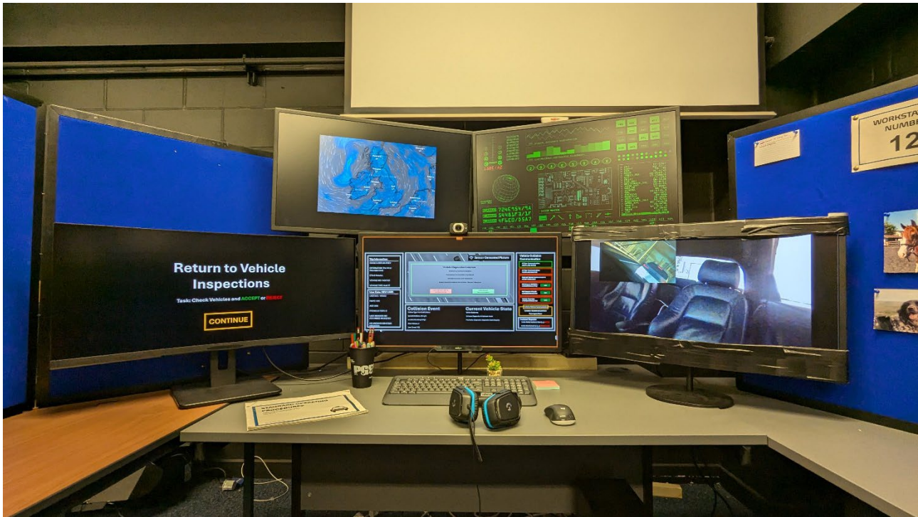
Figure 2: Photo showing the Remote Operation Workstation during a remote operation event (no participant seated in the simulator vehicle), showing on the screens (Top, left to right) weather updates and a generic rolling information screen and (Bottom, left to right) the remote monitoring task, the main remote operation interface and the link to the live view of the road and the user.
