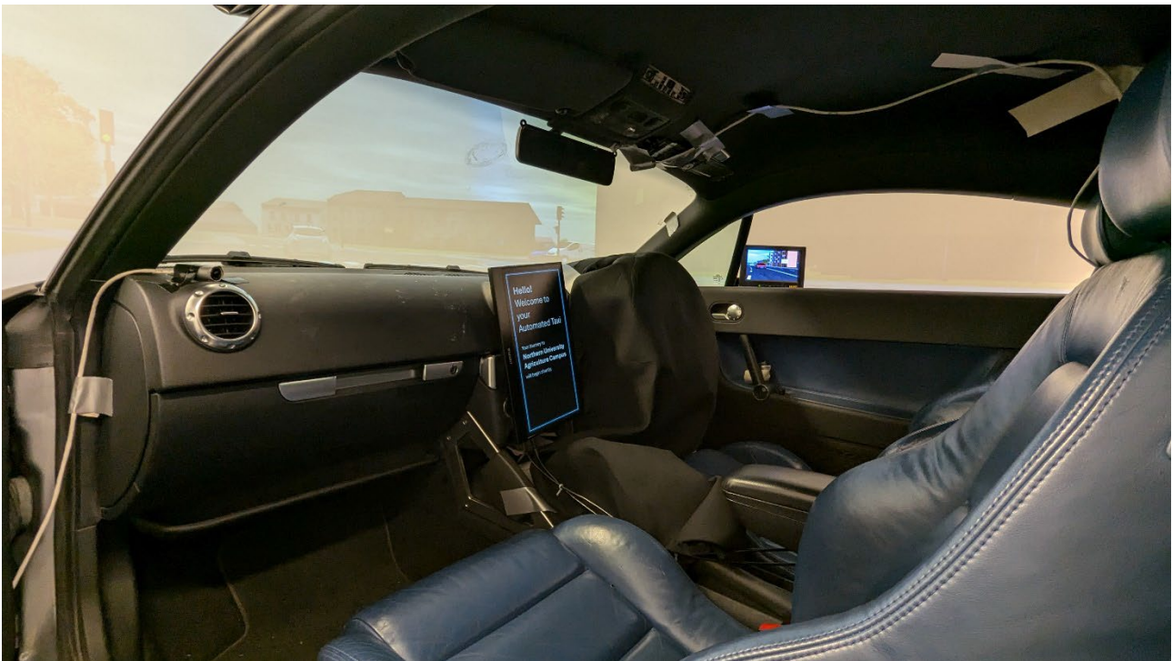
Figure 1: Photo showing the simulator vehicle set-up used during the study. The driving mechanisms (steering wheels, pedals, gearstick and handbrake) are hidden from the participant seated in the front passenger seat.
